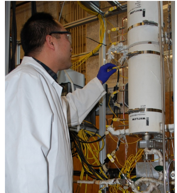
Fixed bed catalytic syngas reactor at Iowa State University
