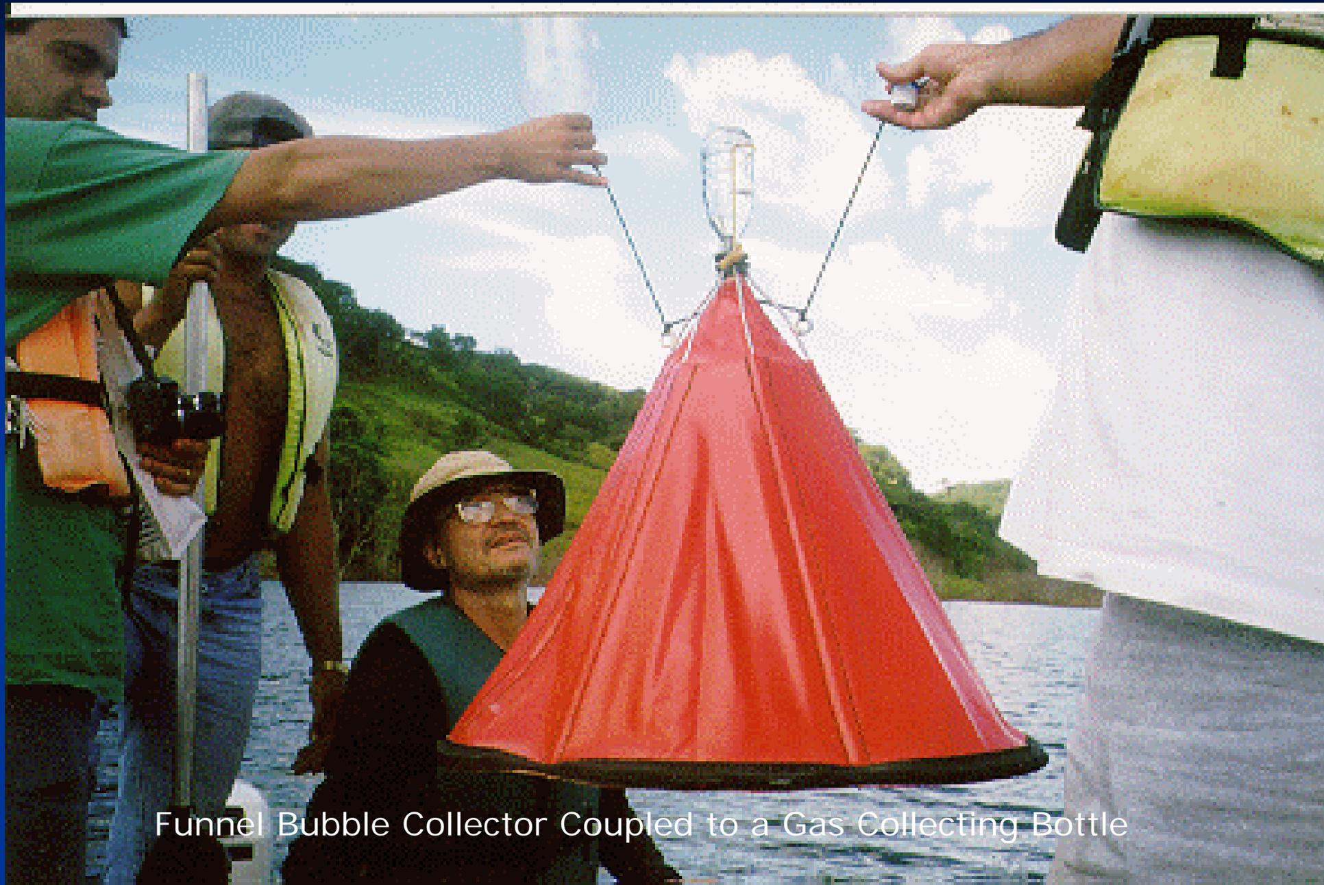
Funnel Bubble Collector Coupled to a Gas Collecting Bottle
