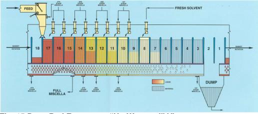
The following Figure 15 shows a horizontal or "un-wrapped view of the Deep Bed Extractor.
