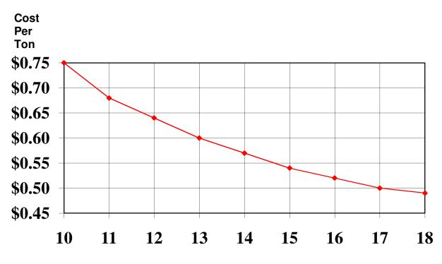
FIG. 09-- Flake Thickness vs. Electrical Cost per Ton
