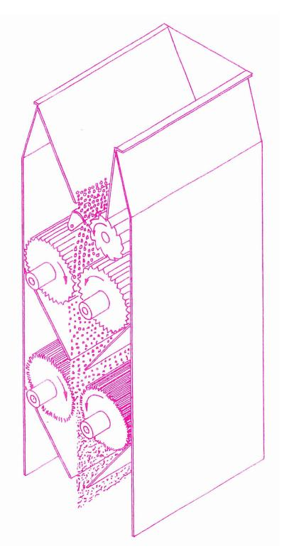
Figure 05—Operation of a Two Pair High Cracking Mill
