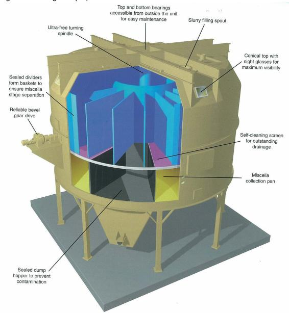
Figure 14—INTERNAL VIEW OF A DEEP BED SOLVENT EXTRACTOR
