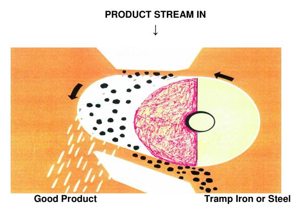
FIG. 03—Rotary Drum Magnet Operation
