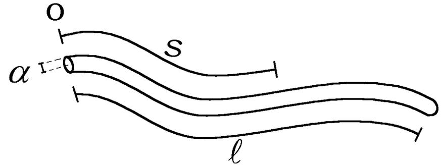
$$\frac{\partial^2 \xi}{\partial s^2} - \frac{1}{c^2} \frac{\partial^2 \xi}{\partial t^2} = \frac{2\pi\epsilon_0 R}{\ell \ln \frac{\ell}{\alpha}} \frac{\partial \xi}{\partial t} \quad \text{onde} \quad \xi = I, \sigma, \phi, A$$
