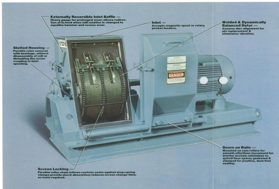
FIG. 19-- Internal View of Hammermill
