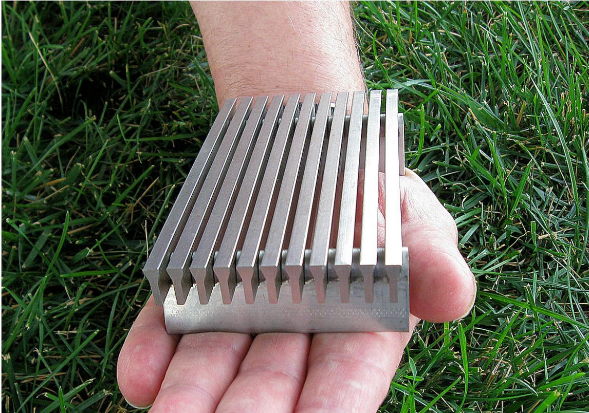
**Fig. 16--Wedge Wire Extractor Bottom**
