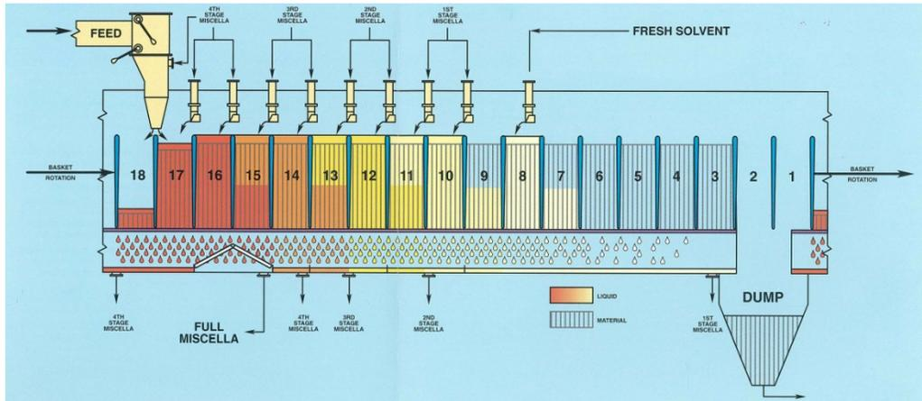
**Fig. 15 Deep Bed Extractor—“Un-Wrapped” View**
