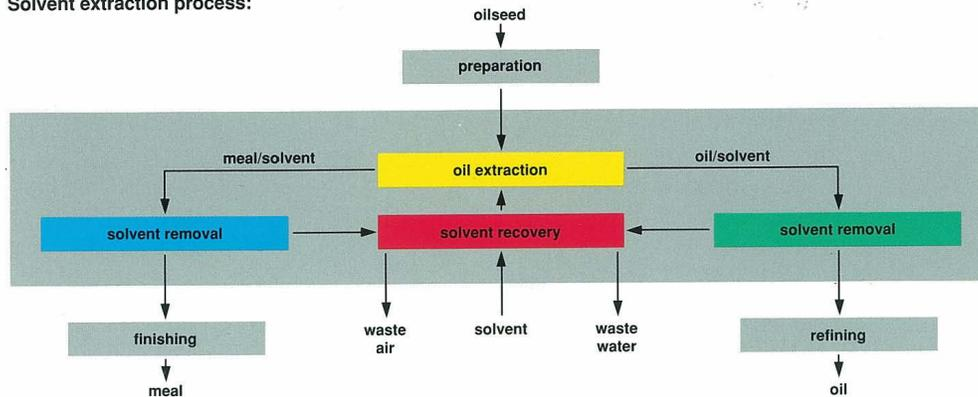
**Diagram 01--The Solvent Extraction Process**
