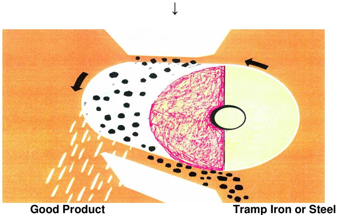
**FIG. 03—Rotary Drum Magnet Operation**
